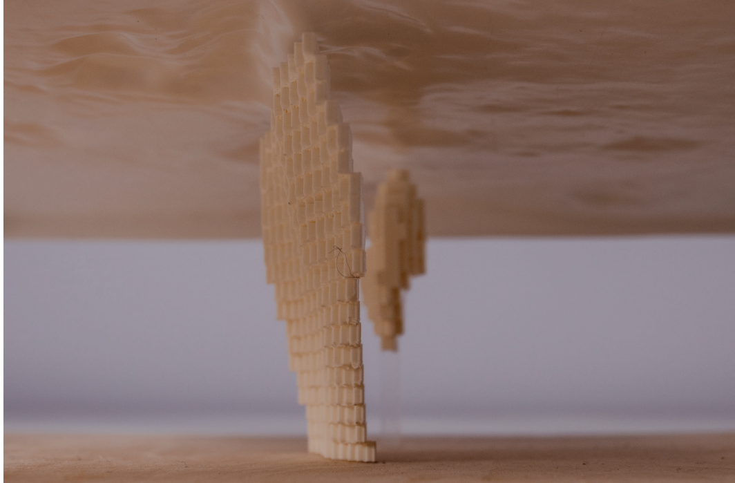
Fig.1: Subterranean model of the Kirunavaara ore body showing the oblique occurrence of the deposit
